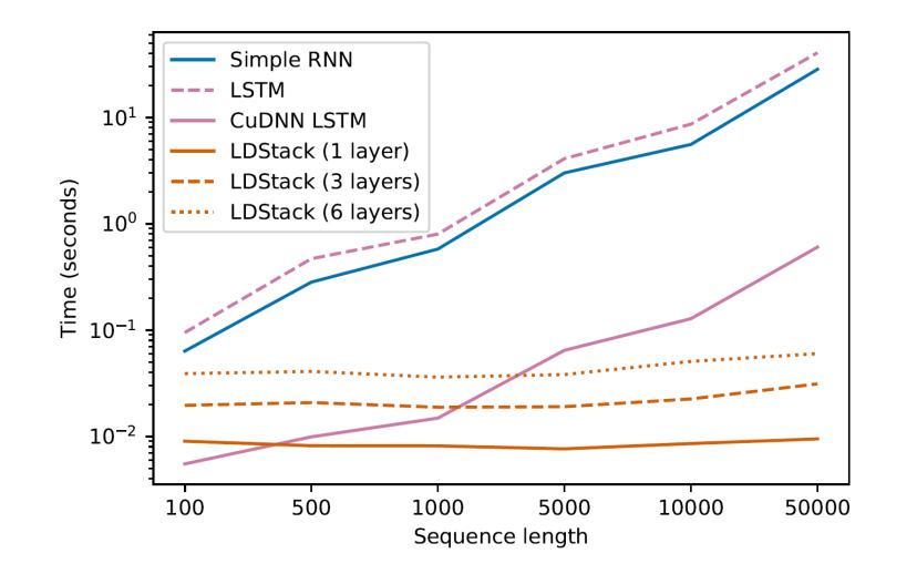
Our construction, called LDStack, is always faster than standard GPU implementations of RNNs. On long sequences, it is even faster than the highly-optimized CuDNN LSTM. We expect these performance results to improve, since our implementation – research code in both Python and CUDA - is not yet optimized.
